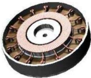
Fig. 1: Impulse magnetisation tool with equal pole lengths
